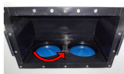
4. Swivel the paper filter anticlockwise.
