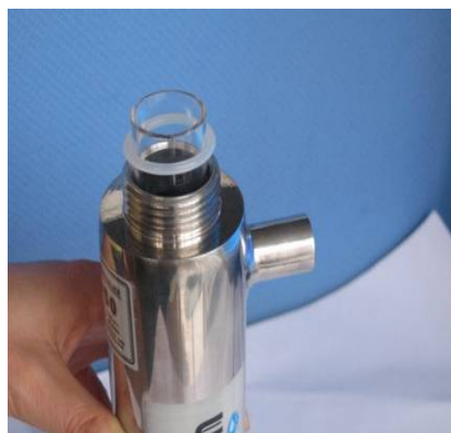
2. Put the O-ring on the quartz sleeve
