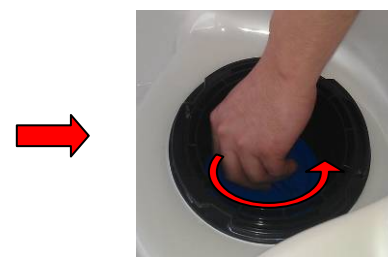
4. Swivel the paper filter anticlockwise.
